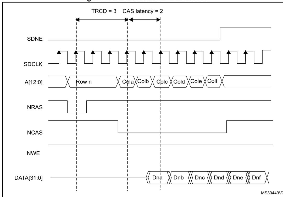
The FMC SDRAM controller features a Cacheable read FIFO (6 lines x 32 bits). It is used to store data read in advance during the CAS latency period and during the RPIPE delay. The following the formula is applied:
