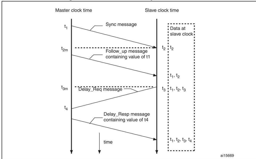
1. The master broadcasts PTP Sync messages to all its nodes. The Sync message contains the master's reference time information. The time at which this message leaves the master's system is  $t_1$ . For Ethernet ports, this time has to be captured at the MII.
