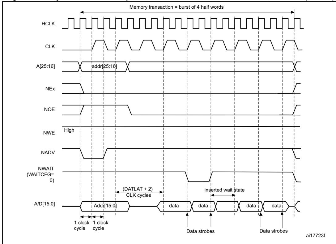
1. Byte lane outputs BL are not shown; for NOR access, they are held high, and, for PSRAM (CRAM) access,
