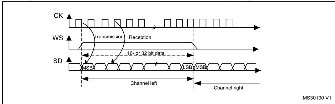
Data are latched on the falling edge of CK (for transmitter) and are read on the rising edge (for the receiver).
