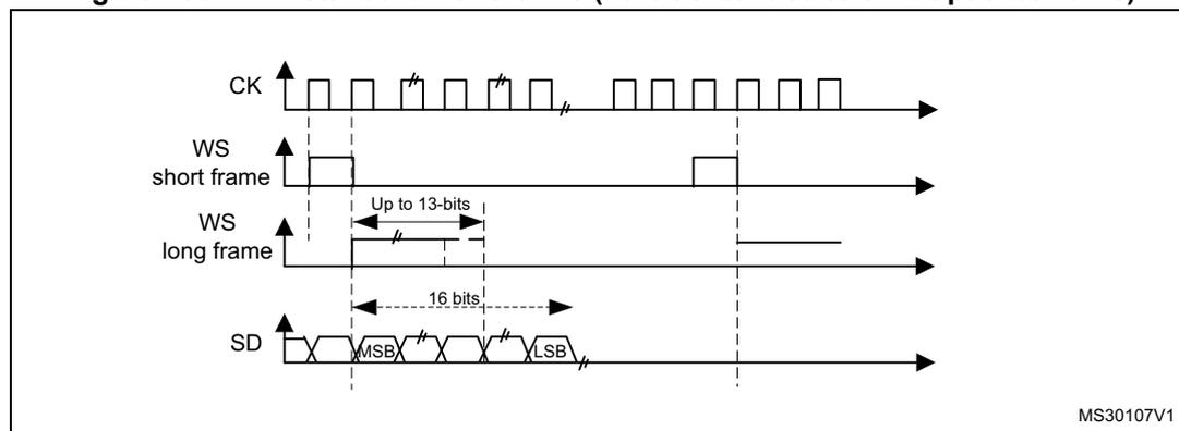
*Note:* For both modes (master and slave) and for both synchronizations (short and long), the number of bits between two consecutive pieces of data (and so two synchronization signals) needs to be specified (DATLEN and CHLEN bits in the SPI\_I2SCFGR register) even in slave mode.
