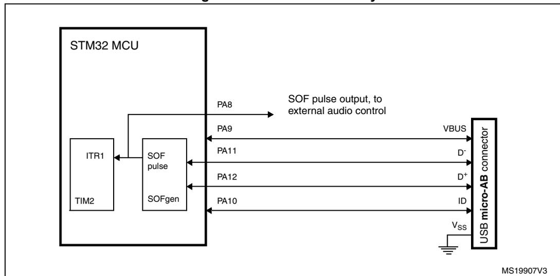
The OTG FS core provides means to monitor, track and configure SOF framing in the host and peripheral, as well as an SOF pulse output connectivity feature.
