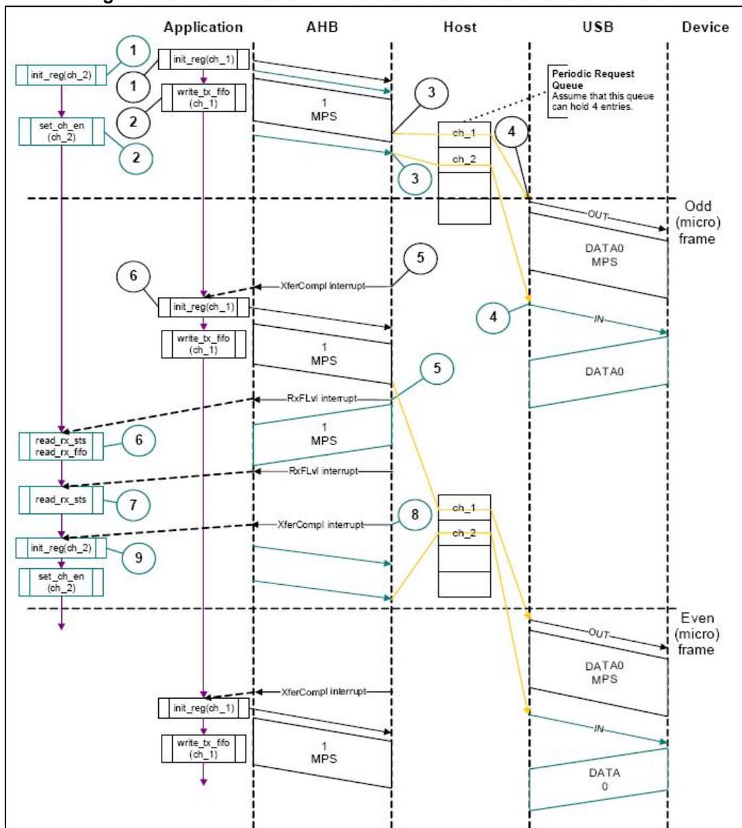
• Interrupt service routine for isochronous OUT/IN transactions
