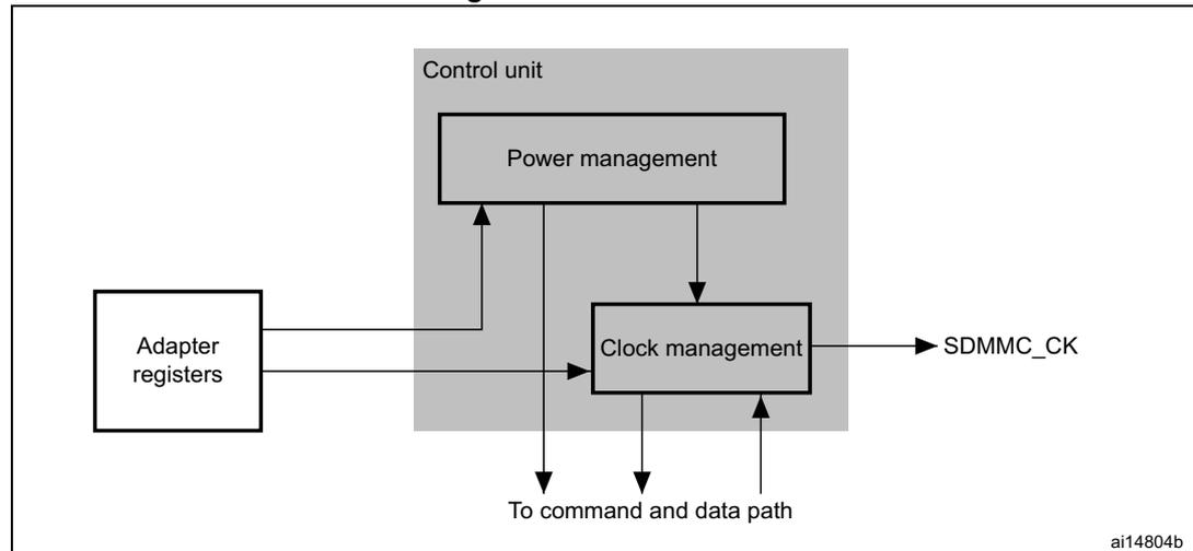
The control unit is illustrated in [Figure 328](#). It consists of a power management subunit and a clock management subunit.
