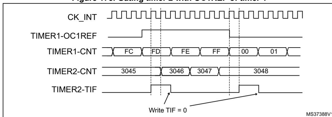
In the example in [Figure 175](#), the Timer 2 counter and prescaler are not initialized before being started. So they start counting from their current value. It is possible to start from a given value by resetting both timers before starting Timer 1. You can then write any value
