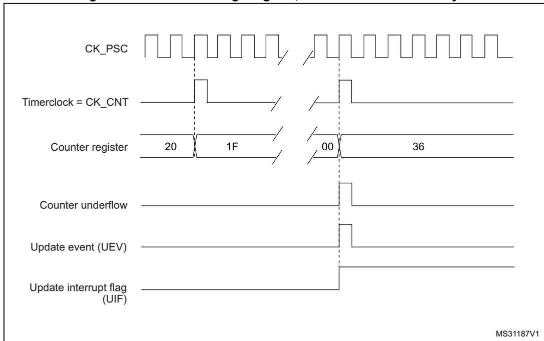
Figure 99. Counter timing diagram, update event when repetition counter is not used
