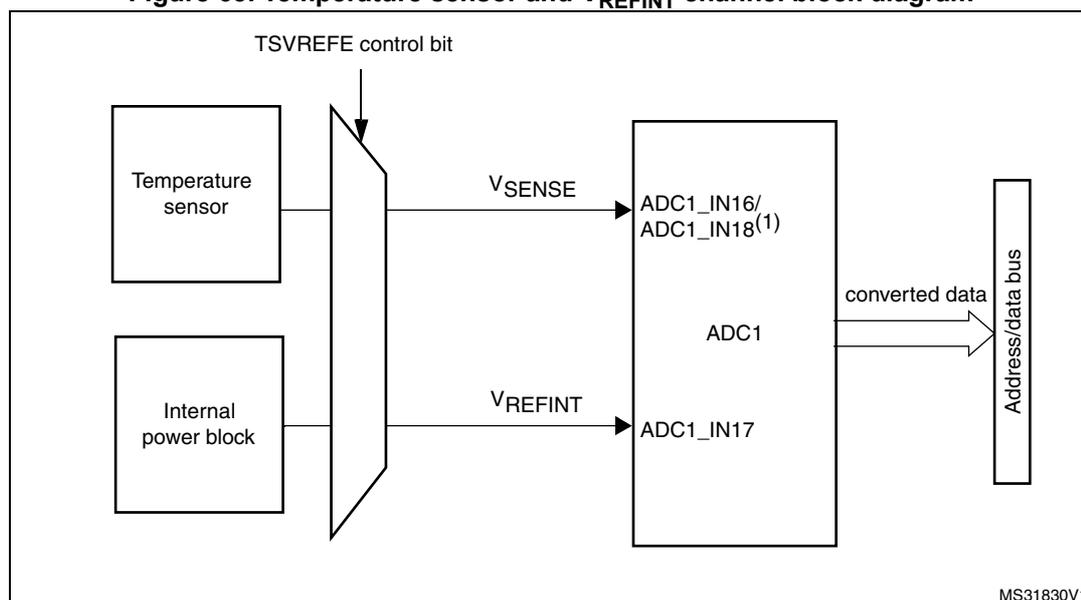
1.  $V_{SENSE}$  is input to ADC1\_IN16 for the STM23F40x and STM32F41x devices and to ADC1\_IN18 for the STM32F42x and STM32F43x devices.
