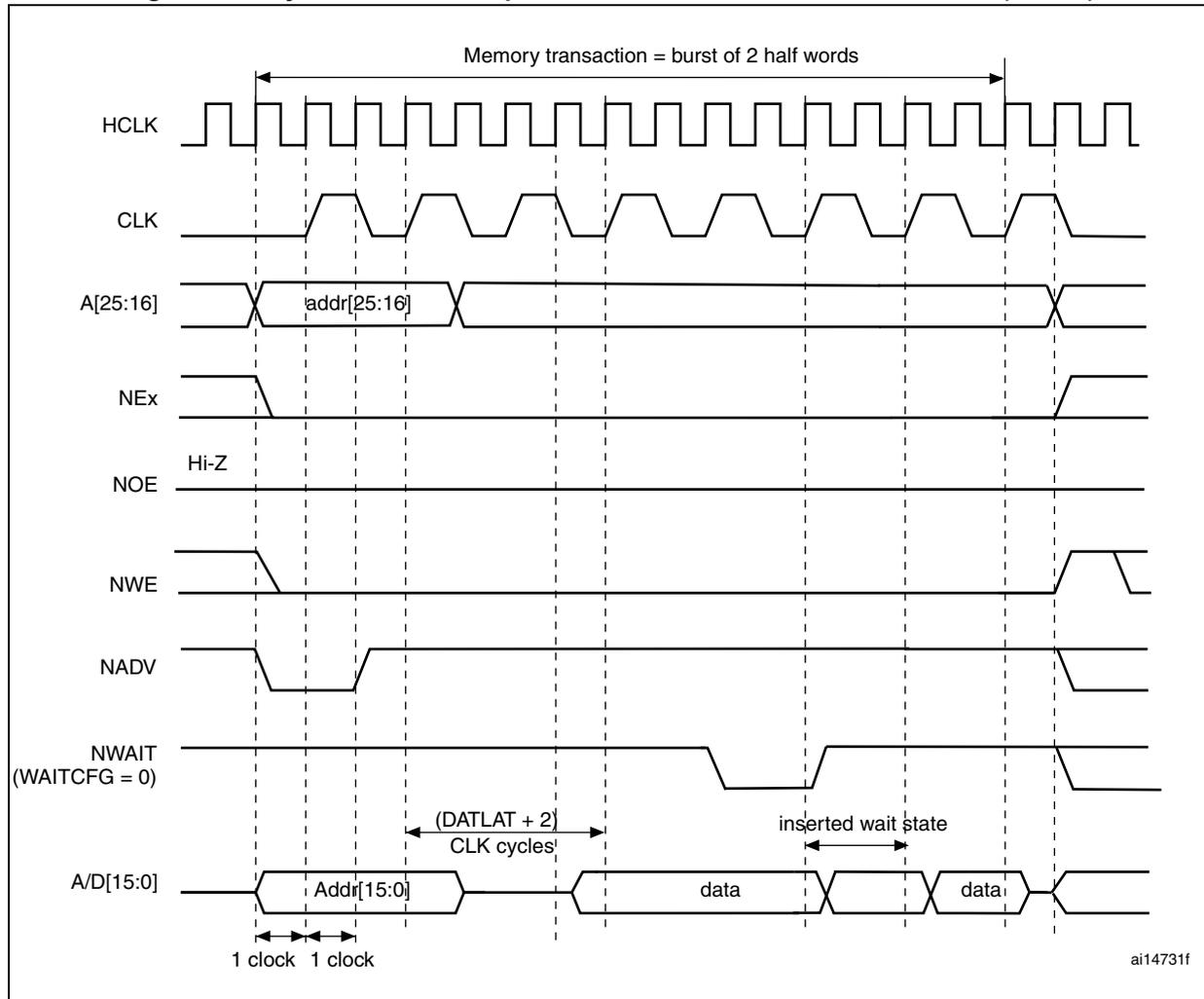
1. The memory must issue NWAIT signal one cycle in advance, accordingly WAITCFG must be programmed to 0.
