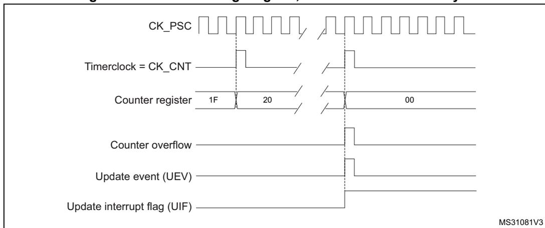
**Figure 93. Counter timing diagram, update event when ARPE=0 (TIMx\_ARR not preloaded)**
