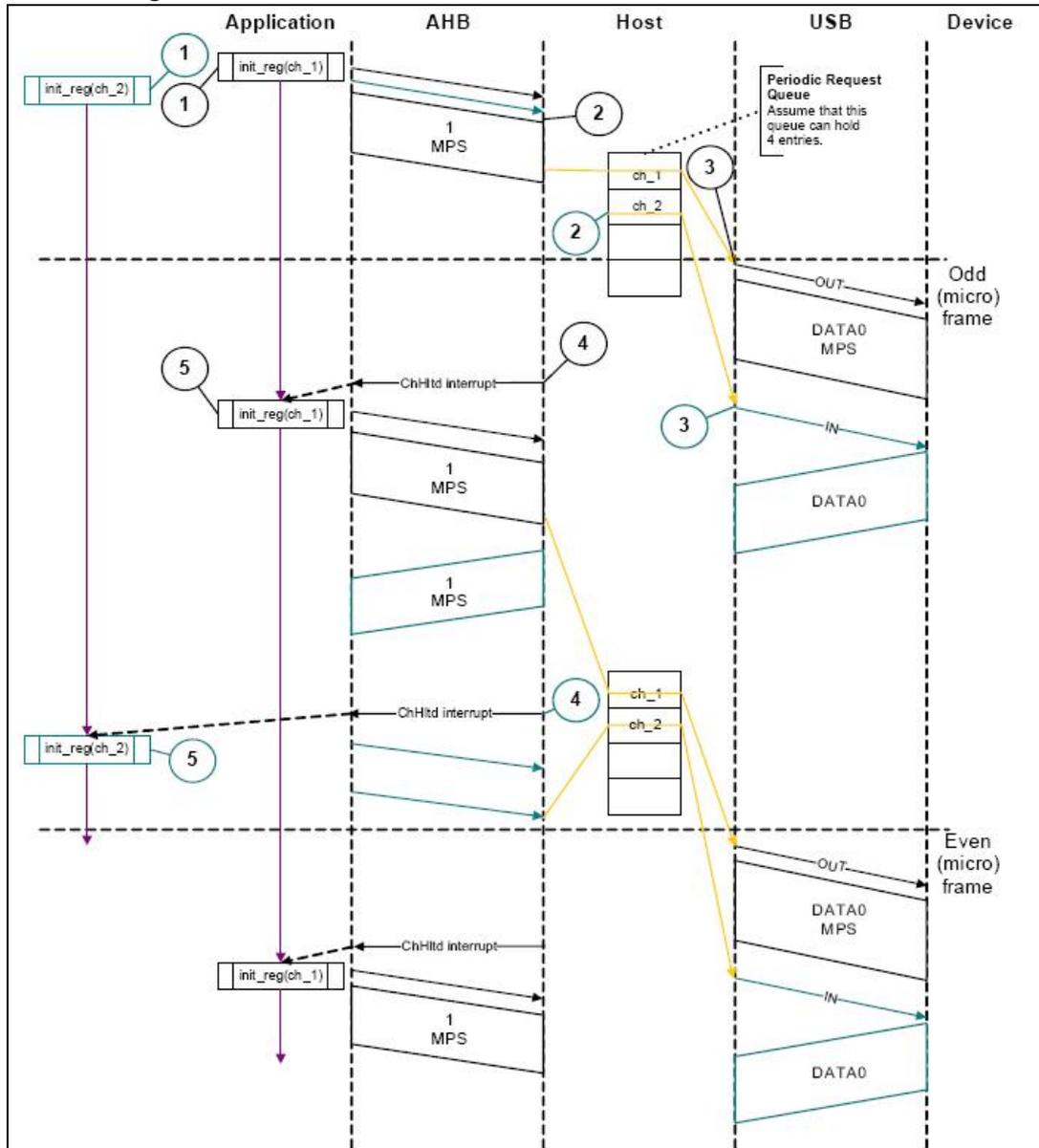
Figure 423. Normal isochronous OUT/IN transactions - Slave mode
