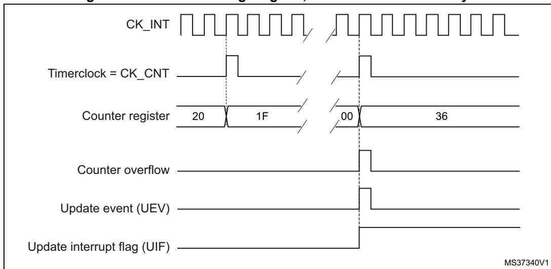
Figure 147. Counter timing diagram, Update event
