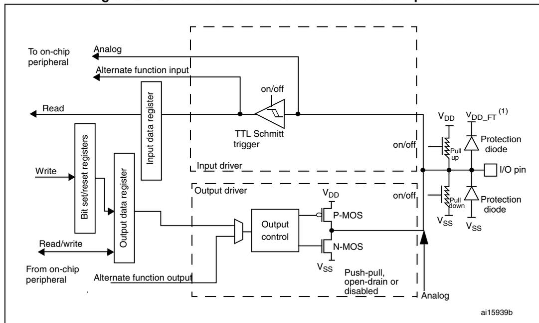
1.  $V_{DD\_FT}$  is a potential specific to five-volt tolerant I/Os and different from  $V_{DD}$ .
