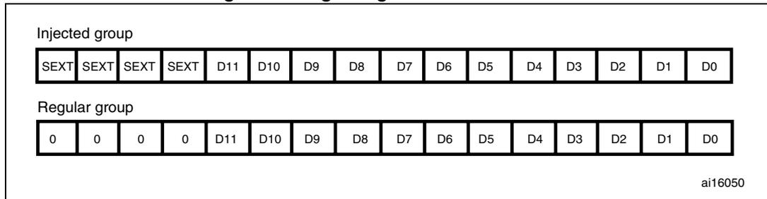
**Figure 49. Left alignment of 12-bit data**
