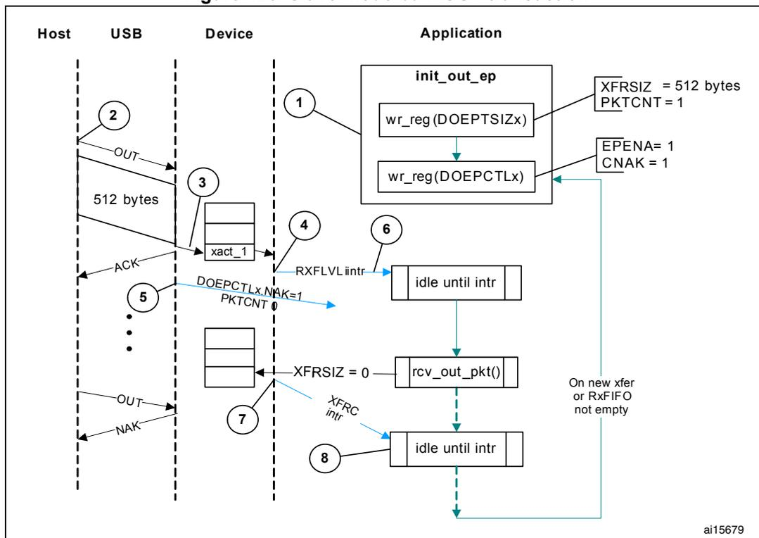
After a SetConfiguration/SetInterface command, the application initializes all OUT endpoints by setting CNAK = 1 and EPENA = 1 (in OTG\_HS\_DOEPCTLx), and setting a suitable XFRSIZ and PKTCNT in the OTG\_HS\_DOEPSIZx register.
