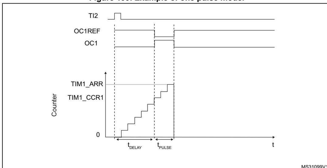
For example the user may want to generate a positive pulse on OC1 with a length of  $t_{\text{PULSE}}$  and after a delay of  $t_{\text{DELAY}}$  as soon as a positive edge is detected on the TI2 input pin.
