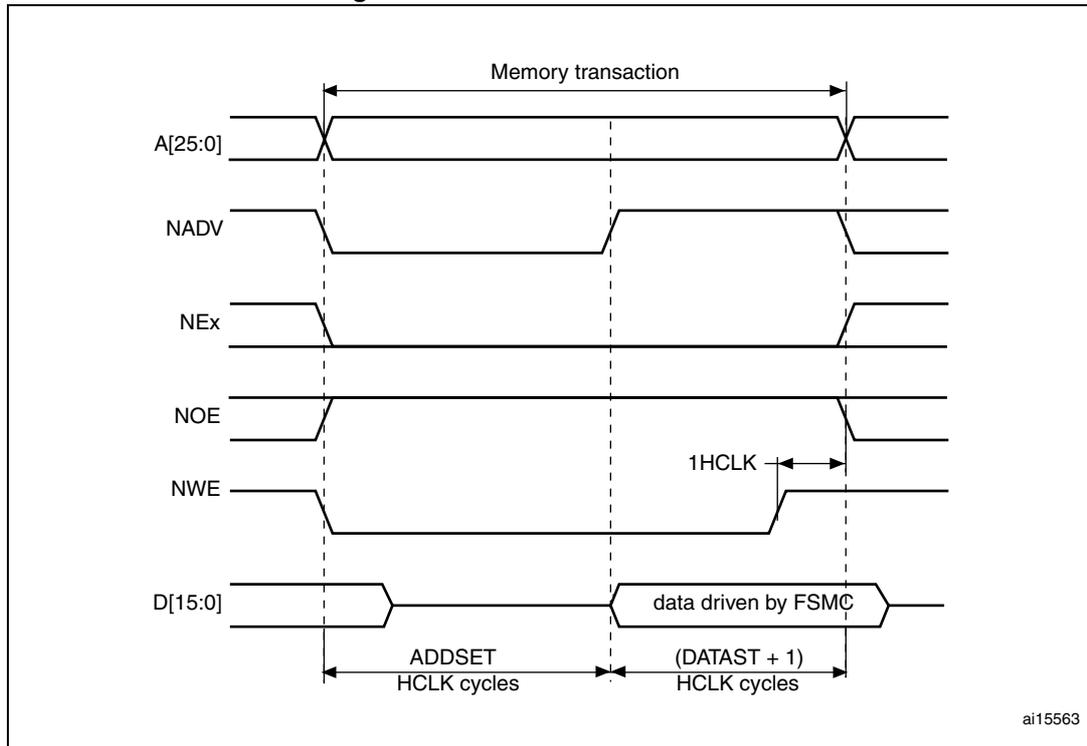
The differences with mode1 are the toggling of NWE and the independent read and write timings when extended mode is set (Mode B).
