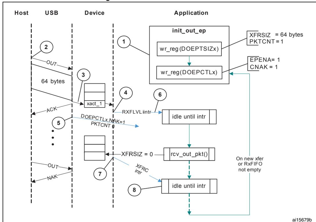
After a SetConfiguration/SetInterface command, the application initializes all OUT endpoints by setting CNAK = 1 and EPENA = 1 (in OTG\_FS\_DOEPCCTLx), and setting a suitable XFRSIZ and PKTCNT in the OTG\_FS\_DOEPTSIZx register.
