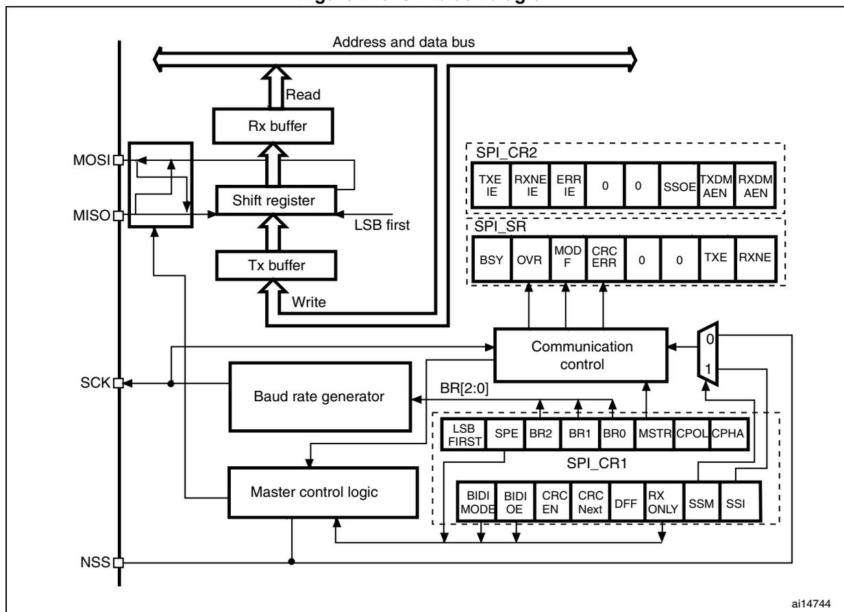
Usually, the SPI is connected to external devices through 4 pins:
