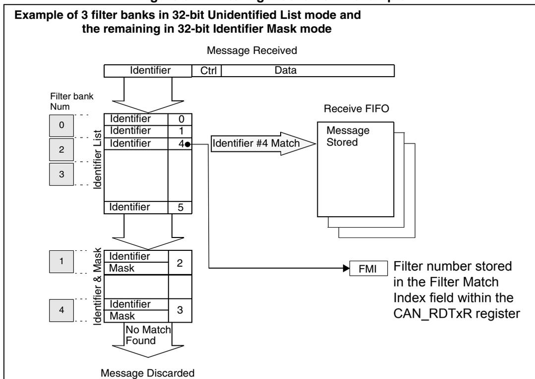
The example above shows the filtering principle of the bxCAN. On reception of a message, the identifier is compared first with the filters configured in identifier list mode. If there is a match, the message is stored in the associated FIFO and the index of the matching filter is stored in the Filter Match Index. As shown in the example, the identifier matches with Identifier #2 thus the message content and FMI 2 is stored in the FIFO.
