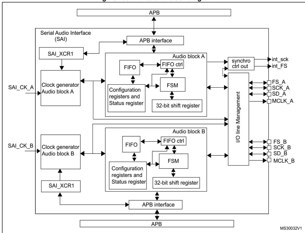
The SAI is mainly composed of two audio sub-blocks with their own clock generator. Each audio block integrates a 32-bit shift register controlled by their own functional state machine. Data are stored or read from the dedicated FIFO. FIFO may be accessed by the CPU, or by DMA in order to leave the CPU free during the communication. Each audio block is independent. They can be synchronous with each other.
