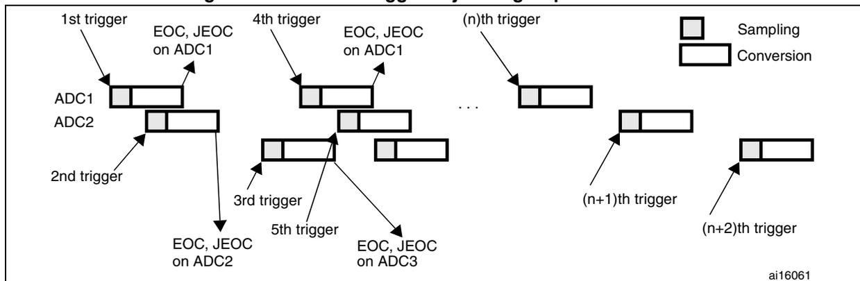
**13.9.5 Combined regular/injected simultaneous mode**
