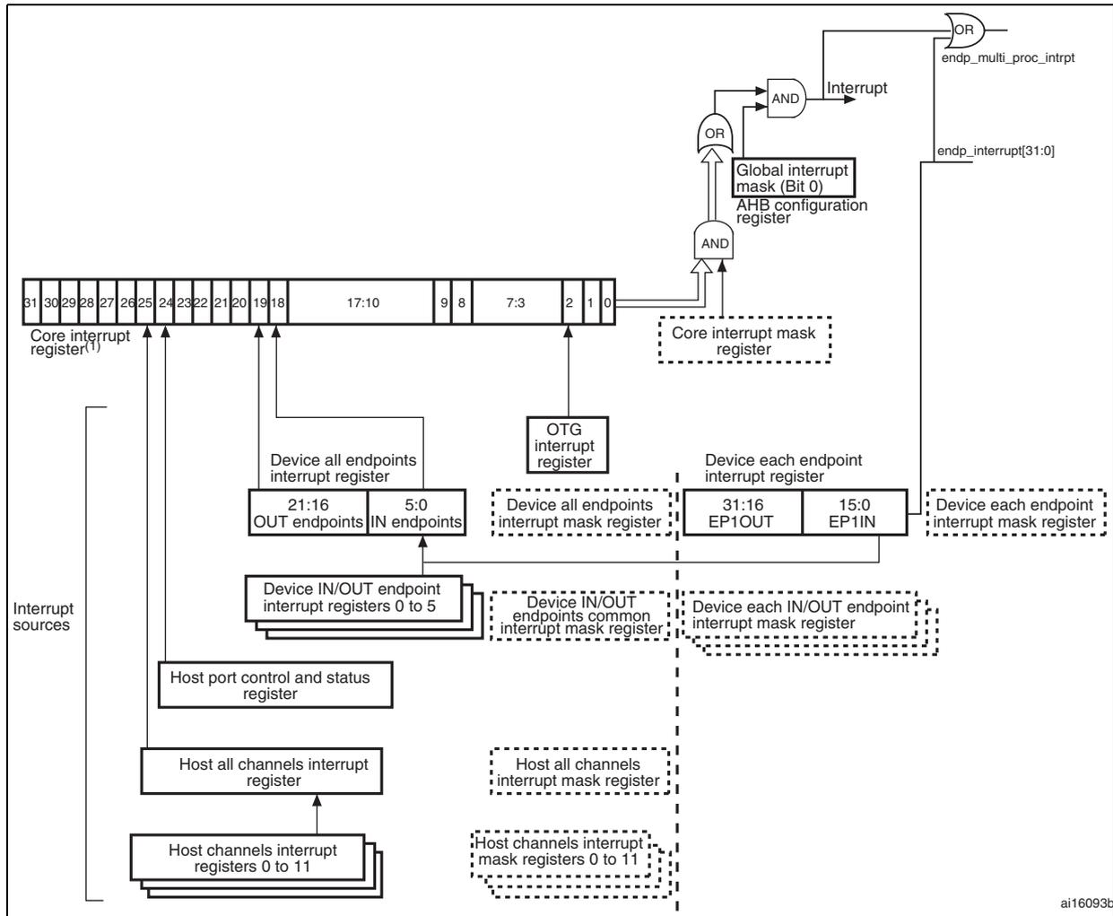
1. The core interrupt register bits are shown in *OTG\_HS core interrupt register (OTG\_HS\_GINTSTS)* on page 1415.
