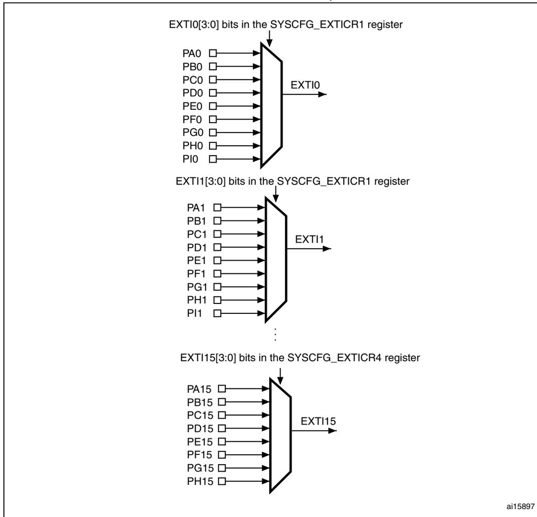
**Figure 43. External interrupt/event GPIO mapping (STM32F42xxx and STM32F43xxx)**
