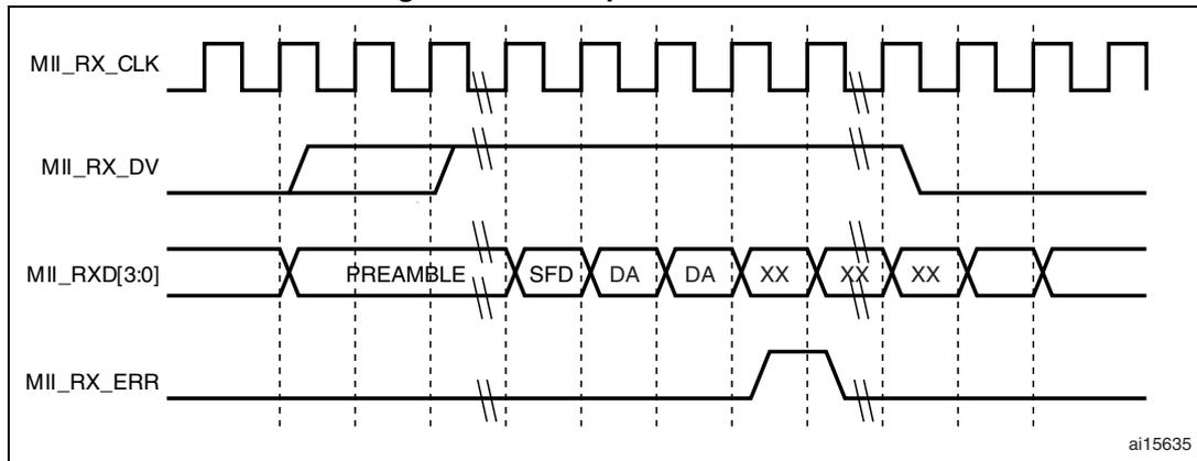
Figure 369. Reception with false carrier indication
