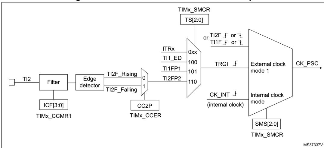
For example, to configure the upcounter to count in response to a rising edge on the TI2 input, use the following procedure:
