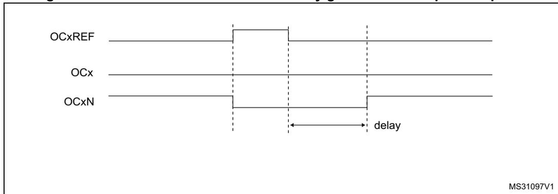
The dead-time delay is the same for each of the channels and is programmable with the DTG bits in the TIMx\_BDTR register. Refer to [Section 17.4.18: TIM1&TIM8 break and dead-time register \(TIMx\\_BDTR\)](#) for delay calculation.
