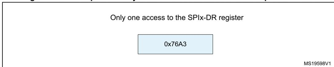
In transmission mode, when TXE is asserted, the application has to write the data to be transmitted (in this case 0x76A3). The 0x000 field is transmitted first (extension on 32-bit). TXE is asserted again as soon as the effective data (0x76A3) is sent on SD.
