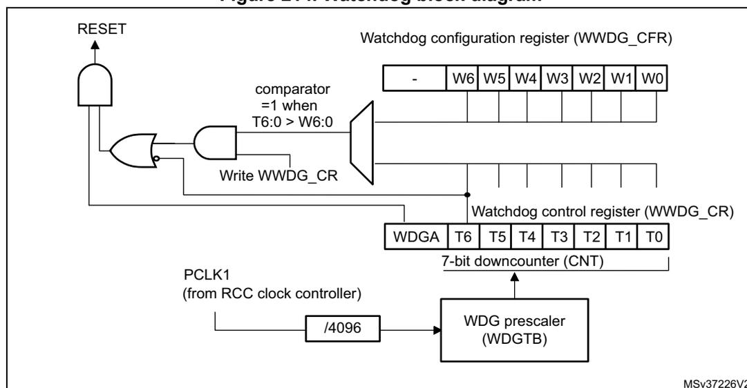
The application program must write in the WWDG\_CR register at regular intervals during normal operation to prevent an MCU reset. This operation must occur only when the counter value is lower than the window register value. The value to be stored in the WWDG\_CR register must be between 0xFF and 0xC0.
