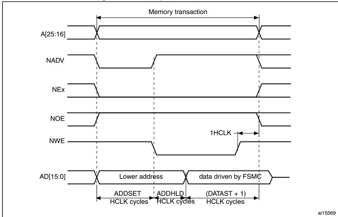
The difference with mode D is the drive of the lower address byte(s) on the databus.
