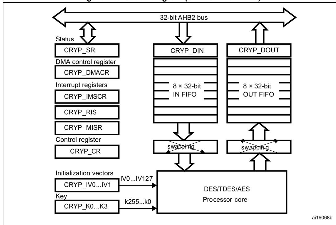
Figure 217. Block diagram (STM32F43xxx)
