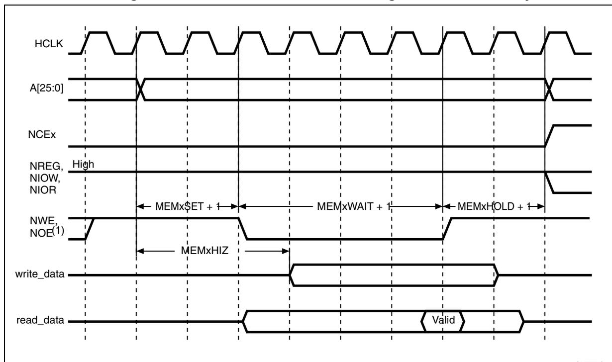
1. NOE remains high (inactive) during write access. NWE remains high (inactive) during read access.
