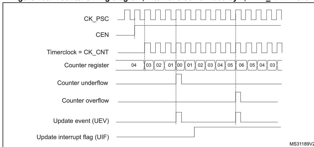
1. Here, center-aligned mode 1 is used (for more details refer to [Section 17.4: TIM1&TIM8 registers](#)).
