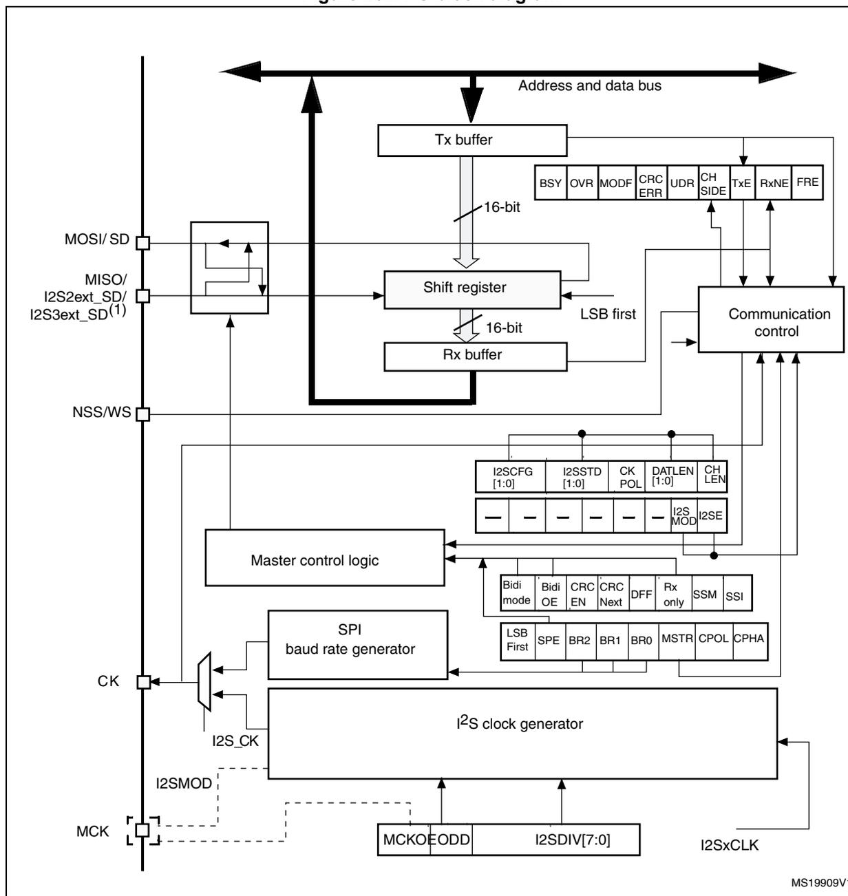
1. I2S2ext\_SD and I2S3ext\_SD are the extended SD pins that control the I<sup>2</sup>S full duplex mode.
