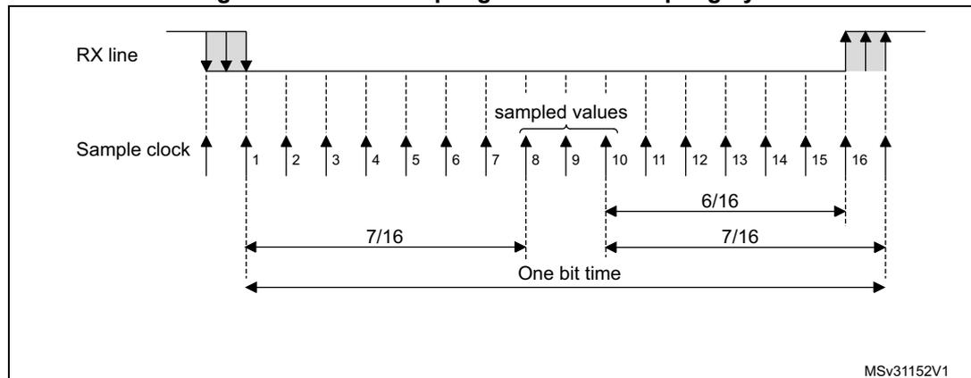
Figure 302. Data sampling when oversampling by 8
