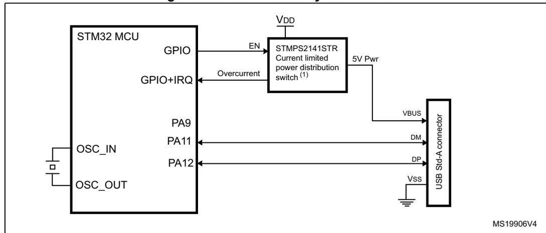
1. STMP2141STR needed only if the application has to support a  $V_{BUS}$  powered device. A basic power switch can be used if 5 V are available on the application board.
