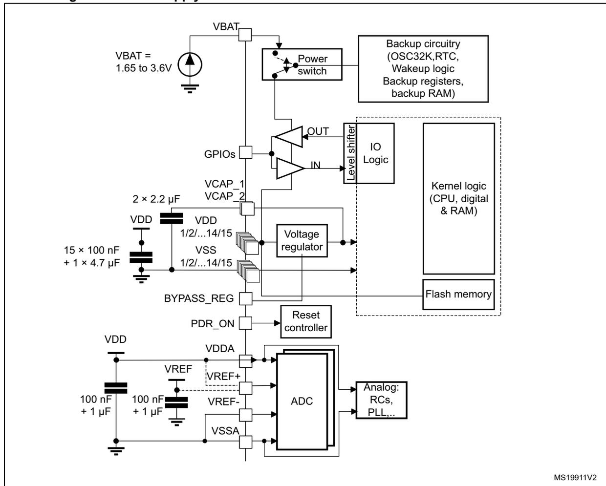
1.  $V_{DDA}$  and  $V_{SSA}$  must be connected to  $V_{DD}$  and  $V_{SS}$ , respectively.
