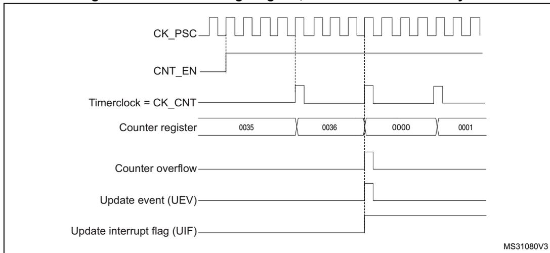
**Figure 92. Counter timing diagram, internal clock divided by N**
