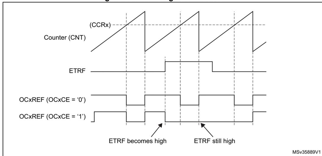
Note: In case of a PWM with a 100% duty cycle (if CCRx>ARR), then OCxREF is enabled again at the next counter overflow.
