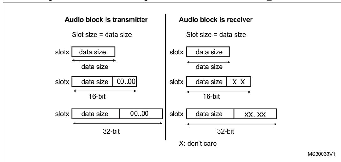
It is possible to choose the position of the first data bit to transfer within the slots, this offset is configured by bit FBOFF[5:0] in the SAI\_xSLOTR register. 0 values will be injected in transmitter mode from the beginning of the slot until this offset position is reached. In reception, the bit in the offset phase is ignored. This feature targets the LSB justified protocol (if the offset is equal to the slot size minus the data size).
