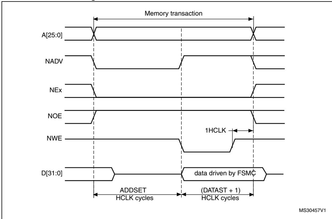
Figure 462. ModeB write access waveforms
