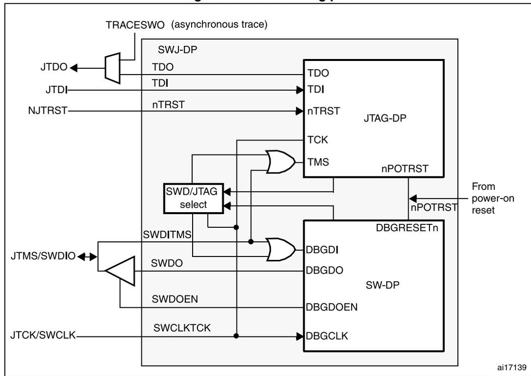
Figure 484 shows that the asynchronous TRACE output (TRACESWO) is multiplexed with TDO. This means that the asynchronous trace can only be used with SW-DP, not JTAG-DP.
