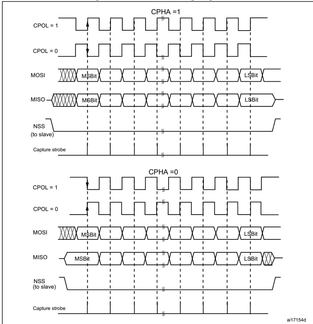
1. These timings are shown with the LSBFIRST bit reset in the SPI\_CR1 register.
