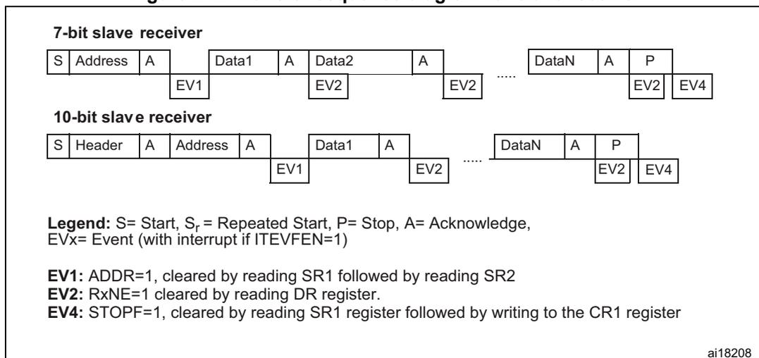
1. The EV1 event stretches SCL low until the end of the corresponding software sequence.
