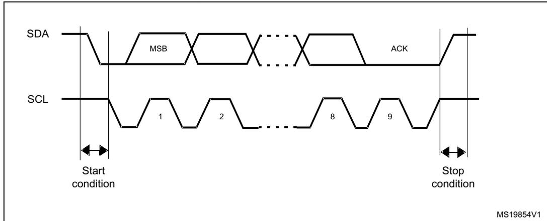
Acknowledge may be enabled or disabled by software. The I<sup>2</sup>C interface addresses (dual addressing 7-bit/ 10-bit and/or general call address) can be selected by software.
