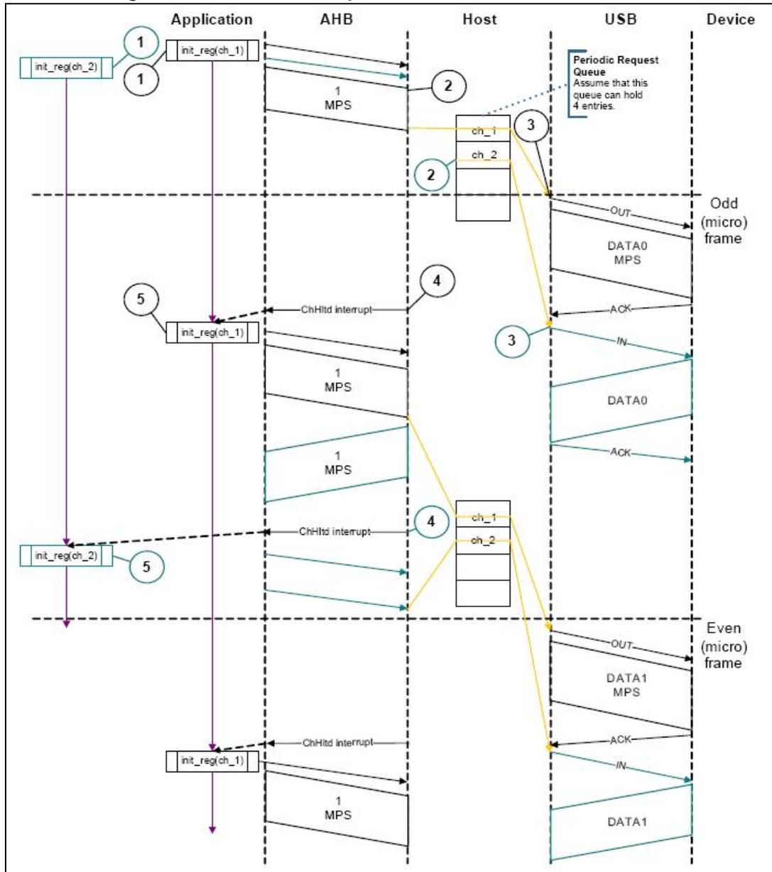
Figure 421. Normal interrupt OUT/IN transactions - Slave mode
