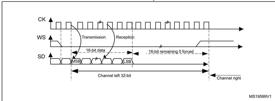
When 16-bit data frame extended to 32-bit channel frame is selected during the I<sup>2</sup>S configuration phase, only one access to SPI\_DR is required. The 16 remaining bits are forced by hardware to 0x0000 to extend the data to 32-bit format.
