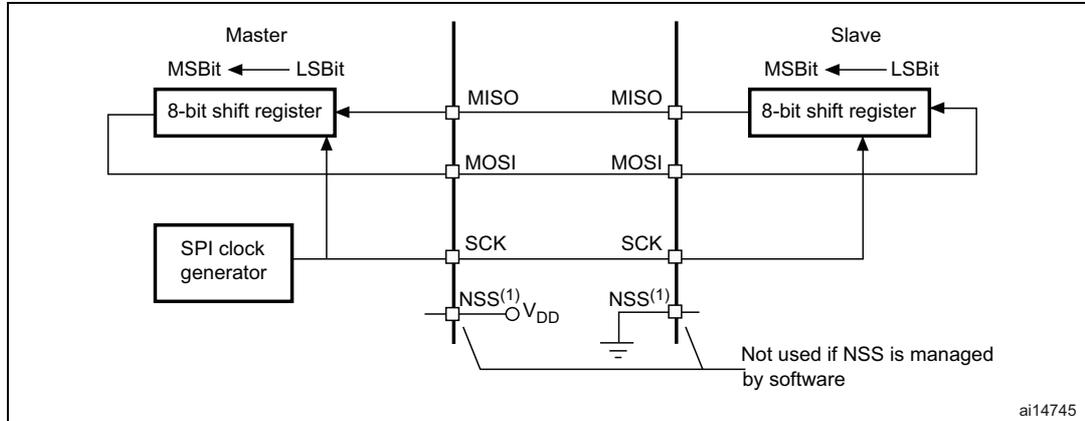
1. Here, the NSS pin is configured as an input.
