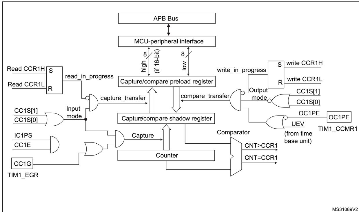
Figure 114. Output stage of capture/compare channel (channel 1 to 3)
