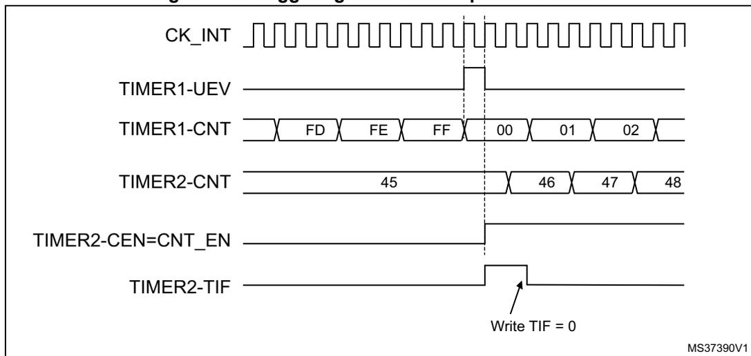
As in the previous example, the user can initialize both counters before starting counting. [Figure 178](#) shows the behavior with the same configuration as in [Figure 177](#) but in trigger mode instead of gated mode (SMS=110 in the TIM2\_SMCR register).
