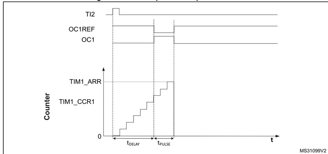
For example the user may want to generate a positive pulse on OC1 with a length of  $t_{PULSE}$  and after a delay of  $t_{DELAY}$  as soon as a positive edge is detected on the TI2 input pin.
