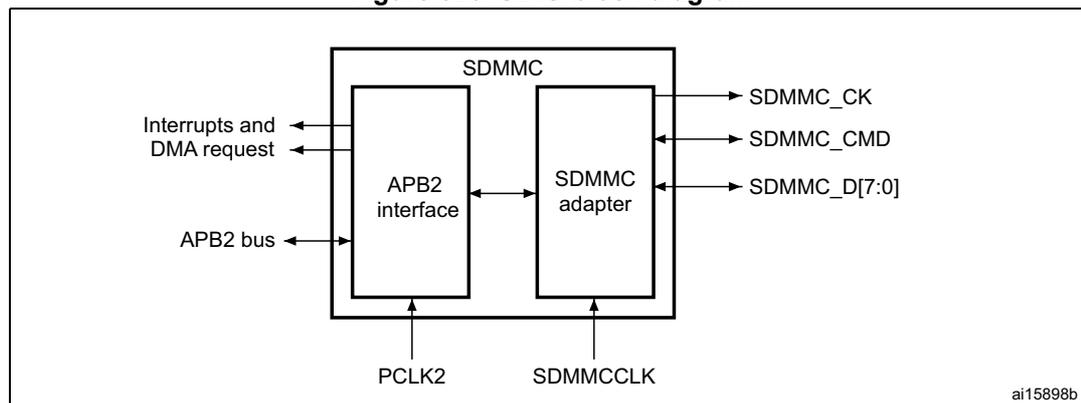
By default SDIO\_D0 is used for data transfer. After initialization, the host can change the databus width.
