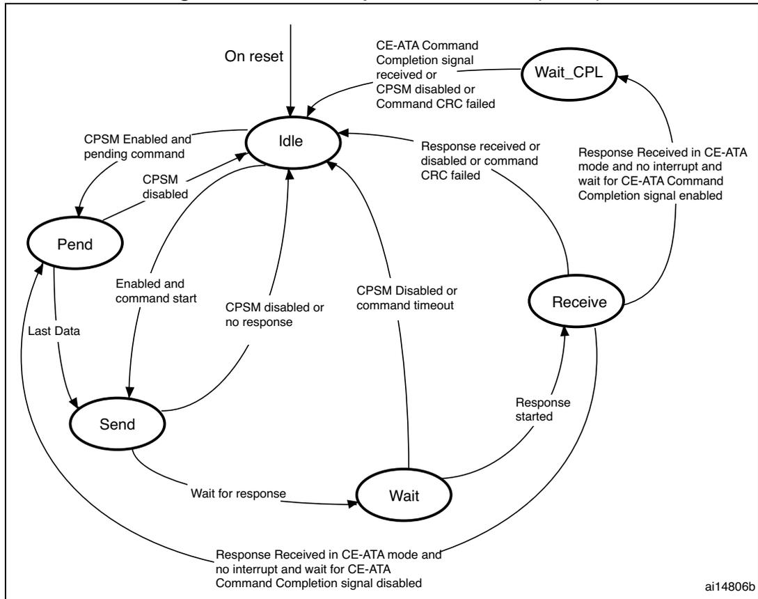
When the Wait state is entered, the command timer starts running. If the timeout is reached before the CPSM moves to the Receive state, the timeout flag is set and the Idle state is entered.
