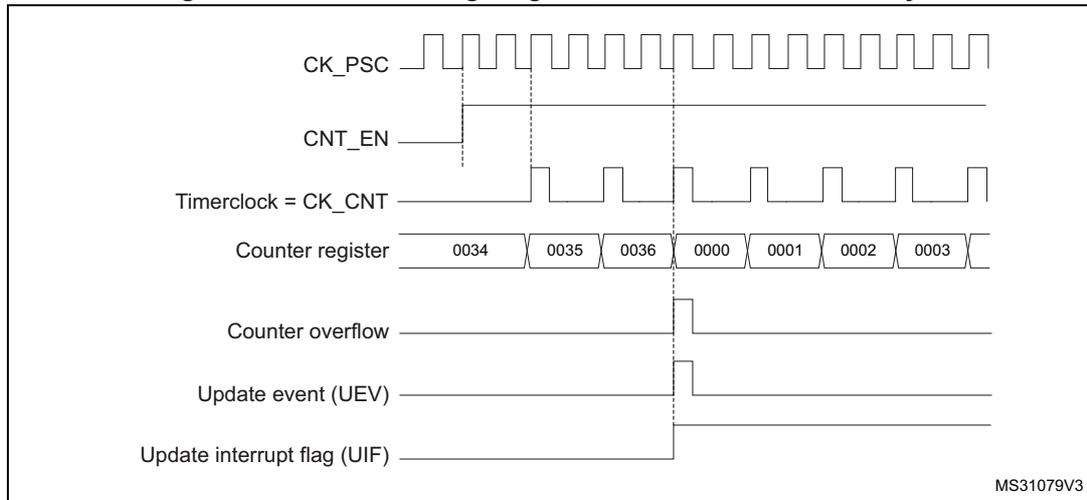
**Figure 91. Counter timing diagram, internal clock divided by 4**
