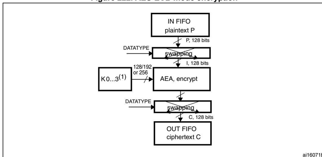
1. K: key; C: cipher text; I: input block; O: output block; P: plain text.
