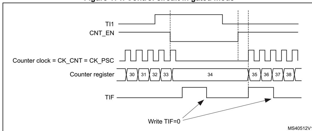
1. The configuration "CCxP=CCxNP=1" (detection of both rising and falling edges) does not have any effect in gated mode because gated mode acts on a level and not on an edge.
