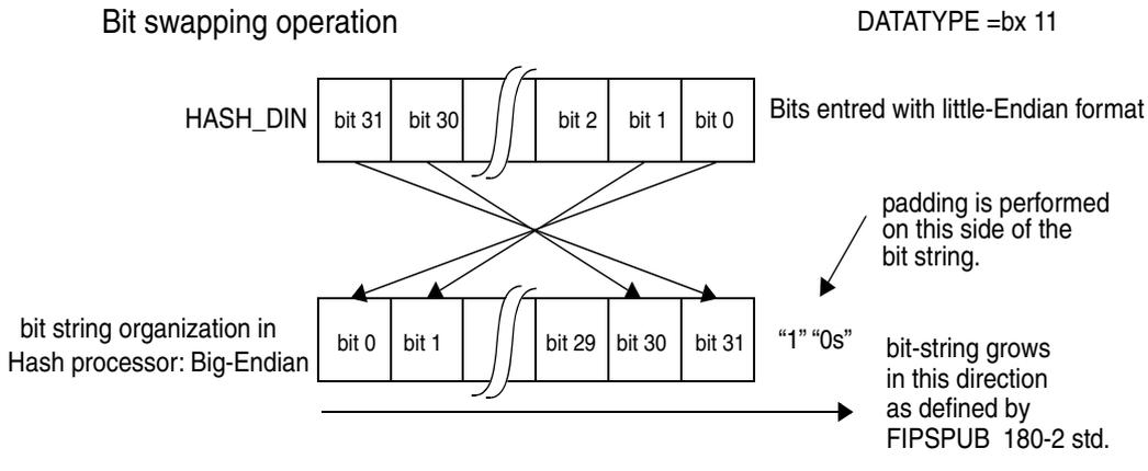
B-In case of byte data hash, all bytes should be swapped as below
