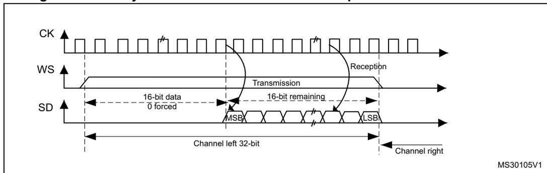
When 16-bit data frame extended to 32-bit channel frame is selected during the I<sup>2</sup>S configuration phase, Only one access to SPI\_DR is required. The 16 remaining bits are forced by hardware to 0x0000 to extend the data to 32-bit format. In this case it corresponds to the half-word MSB.
