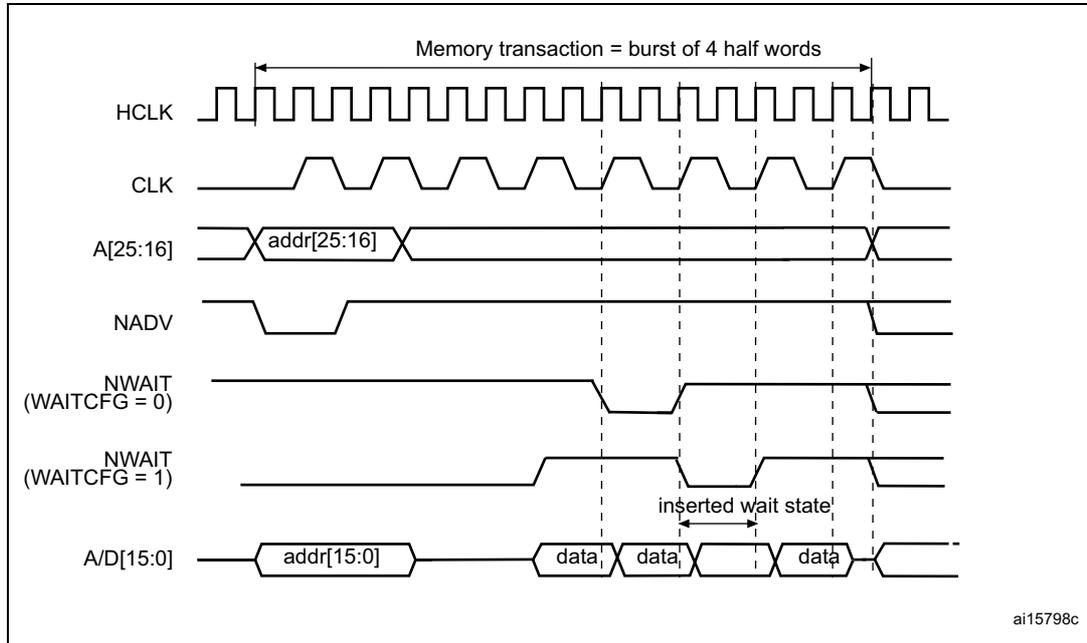
**Figure 472. Synchronous multiplexed read mode waveforms - NOR, PSRAM (CRAM)**
