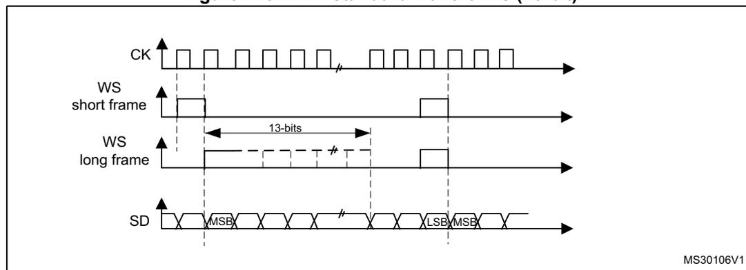
For long frame synchronization, the WS signal assertion time is fixed 13 bits in master mode.
