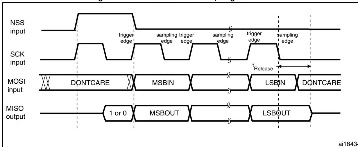
Figure 250. TI mode - Slave mode, continuous transfer
