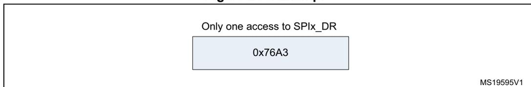
For transmission, each time an MSB is written to SPI\_DR, the TXE flag is set and its interrupt, if allowed, is generated to load SPI\_DR with the new value to send. This takes place even if 0x0000 have not yet been sent because it is done by hardware.
