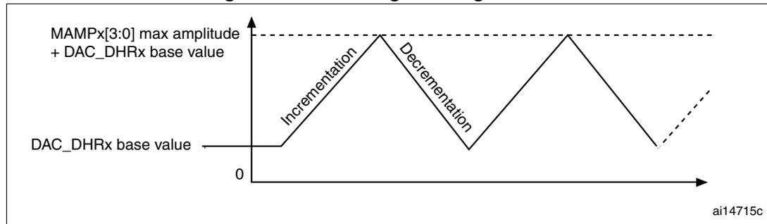
**Figure 71. DAC conversion (SW trigger enabled) with triangle wave generation**
