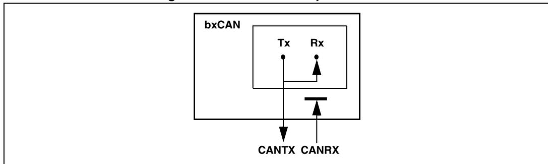
This mode is provided for self-test functions. To be independent of external events, the CAN Core ignores acknowledge errors (no dominant bit sampled in the acknowledge slot of a data / remote frame) in Loop Back Mode. In this mode, the bxCAN performs an internal feedback from its Tx output to its Rx input. The actual value of the CANRX input pin is disregarded by the bxCAN. The transmitted messages can be monitored on the CANTX pin.
