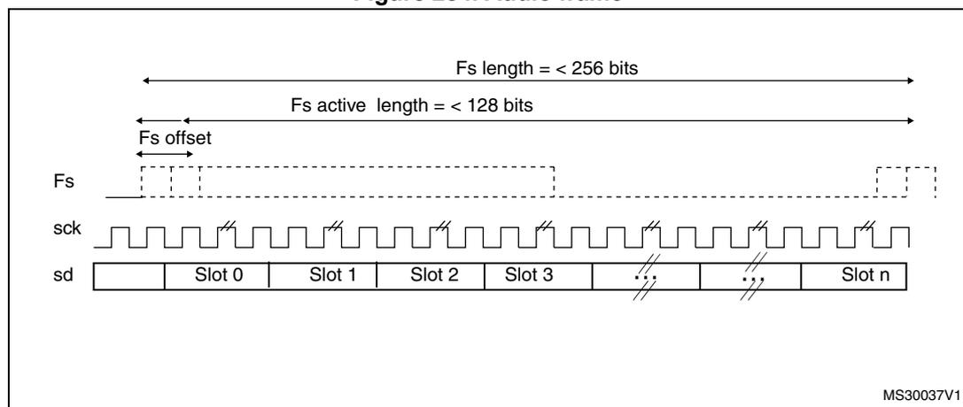
In AC'97 mode (bit PRTCFG[1:0] = 10 in the SAI\_xCR1 register), the frame synchronization shape is forced to be configured to target these protocols. The SAI\_xFRCR register value is ignored.
