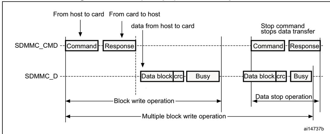
Note: The SDIO will not send any data as long as the Busy signal is asserted (SDIO\_D0 pulled low).
