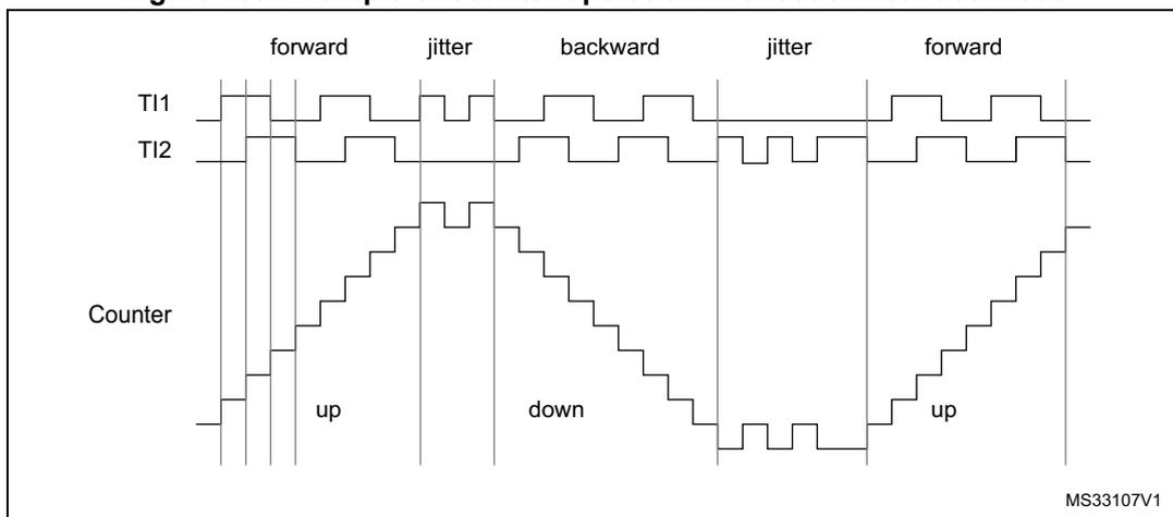
Figure 169 gives an example of counter behavior when TI1FP1 polarity is inverted (same configuration as above except CC1P=1).
