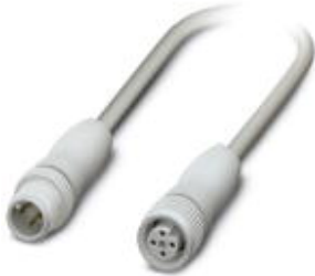
Sensor/Actuator cable, 4-position, PP-EPDM halogen-free, Gray RAL 7035, Plug straight M12, A-coded, on Socket straight M12, A-coded, Cable length: 0.6 m, Hygienic design, with plastic knurl
