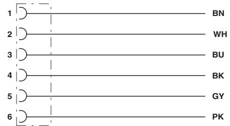
Contact assignment of M8 socket
