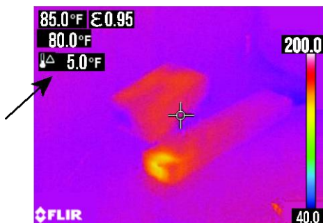
Fig. 8-4 Type-K / IGM Temperature Differential Reading Example
