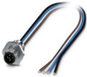
Flush-type connector, Power, 4-position, Plug, Link: M12, T power, Front mounting, M16 x 1.5, Individual wires, Cable length: 0.5 m
