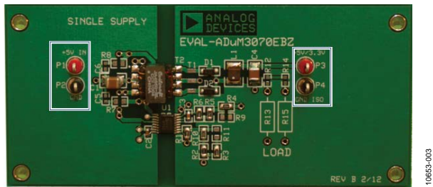
Figure 3. Single Supply Terminals
