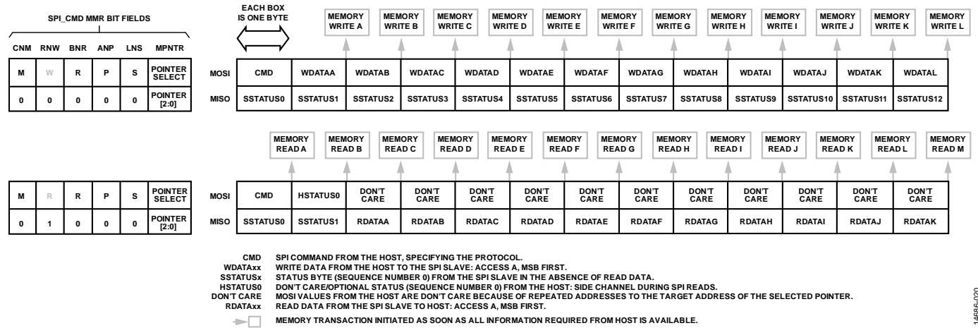
Figure 19. Memory Write/Read, Random, Pointer, Short Address
