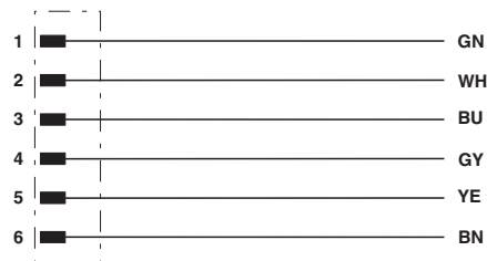
Contact assignment of 7/8" plug
