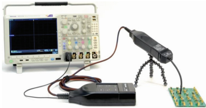
Figure 4: Tektronix IsoVu measurement setup.
