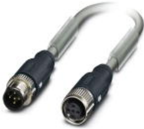
Bus system cable, CANopen®, 5-position, PUR halogen-free, Gray RAL 7001, shielded, Plug straight M12-SPEEDCON, A-coded, on Socket straight M12-SPEEDCON, A-coded, Cable length: 15 m
