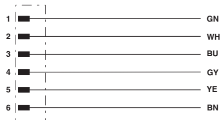
Contact assignment of 7/8" plug
