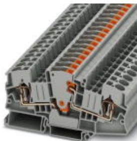
Test disconnect terminal block, Connection method: Spring-cage connection, Cross section: 0.2 mm 2 - 10 mm 2 , AWG: 24 - 10, Width: 8.2 mm, Color: gray
