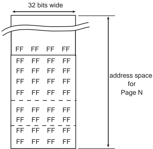
Step 1: Flash array after page erase
