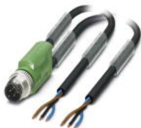
Sensor/actuator cable, 3-position, PUR halogen-free, black-gray RAL 7021, Plug straight M12, A-coded, on free cable end and free cable end, cable length: 3 m
