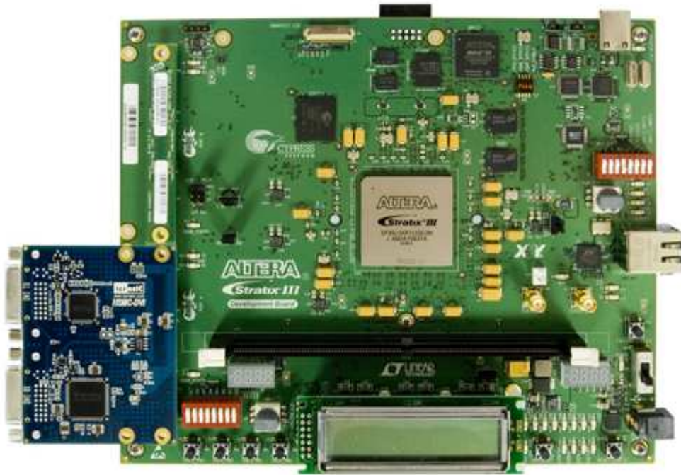
Figure 1.2.5. The HSMC-DVI board connects with Stratix III Development Board
