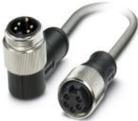
Bus system cable, DeviceNet, 5-position, PUR halogen-free, Gray RAL 7001, Plug angled 7/8"-16UNF, on Socket straight 7/8"-16UNF, Cable length: 15 m
