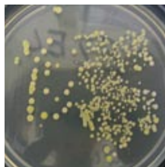
Bacteria growth on ordinary sensor after 12 hours.
